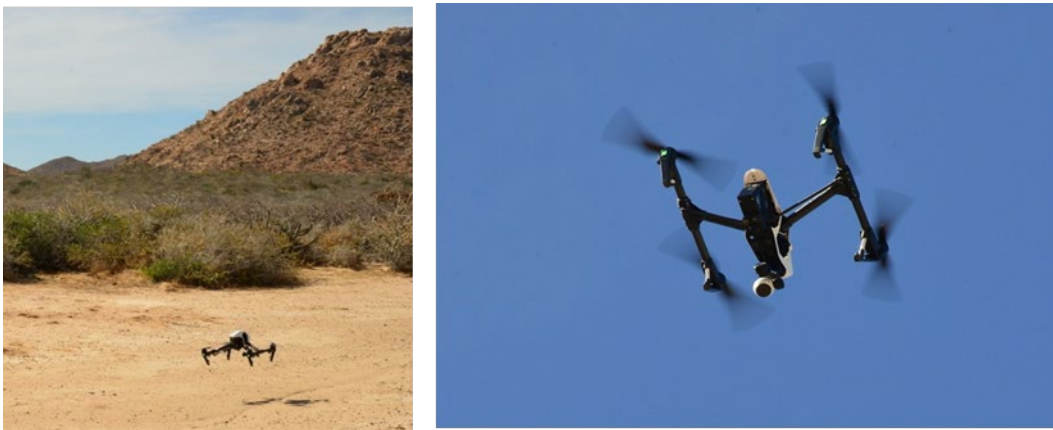
Figure 2. Left: Take-off from an Inspire 1 quadcopter UAV. Right: Inspire 1 in the air conducting an autonomous flight mission.
